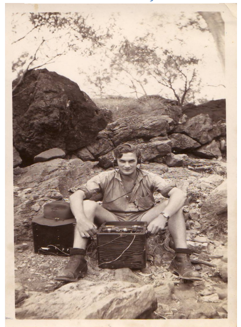
(Bob Fry operating his home made Geiger counter in the Mt Painter area of South Australia)
